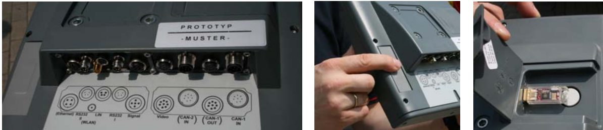
Fig. 3: Hardware of the CCI ISOBUS terminal (examples): interfaces (left), bottom for switching to the one-hand operation mode (center), USB storage
