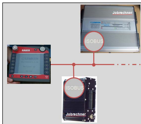
Fig. 1: Cross-manufacturer combination of an SOBUS terminal and control units (ECU)
