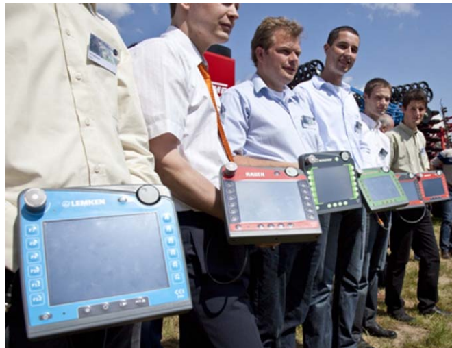
Fig. 4: CCI ISOBUS terminals of the companies Lemken, Rauch, Kuhn, Krone, Amazone and Grimme (same hardware, different foil with corporate design)
